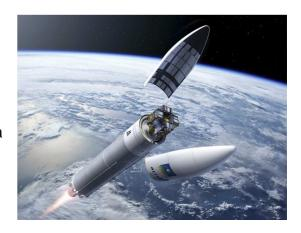
The upper stage – carrying four 715-kg Galileo satellites – will fly in ballistic configuration for three hours and eight minutes, after which a second upper stage firing will place it into circular separation orbit.
